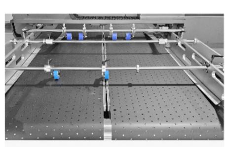
System: Features Automatic Deviation Correction, Strong Platform Adsorption.
