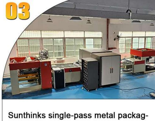
ing printing solutions are centered around automatic control and utilize a four-in-one integrated design encompassing feeding, printing, curing, and stacking. This creates a complete assembly-line operation system that effectively reduces process transition time and optimizes production rhythm.
